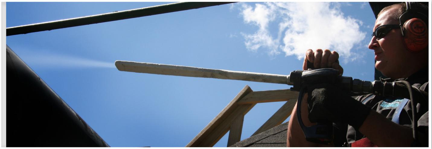
*"WE WERE ABLE TO GET ON TOP OF WHEELS, IN CORNERS AND OTHER TIGHT PLACES WITH THE DRY ICE BLASTING SYSTEM THAT HAD NOT PREVIOUSLY BEEN CLEANED, REMOVING LAYERS OF PAINT, GREASE AND DIRT."*
